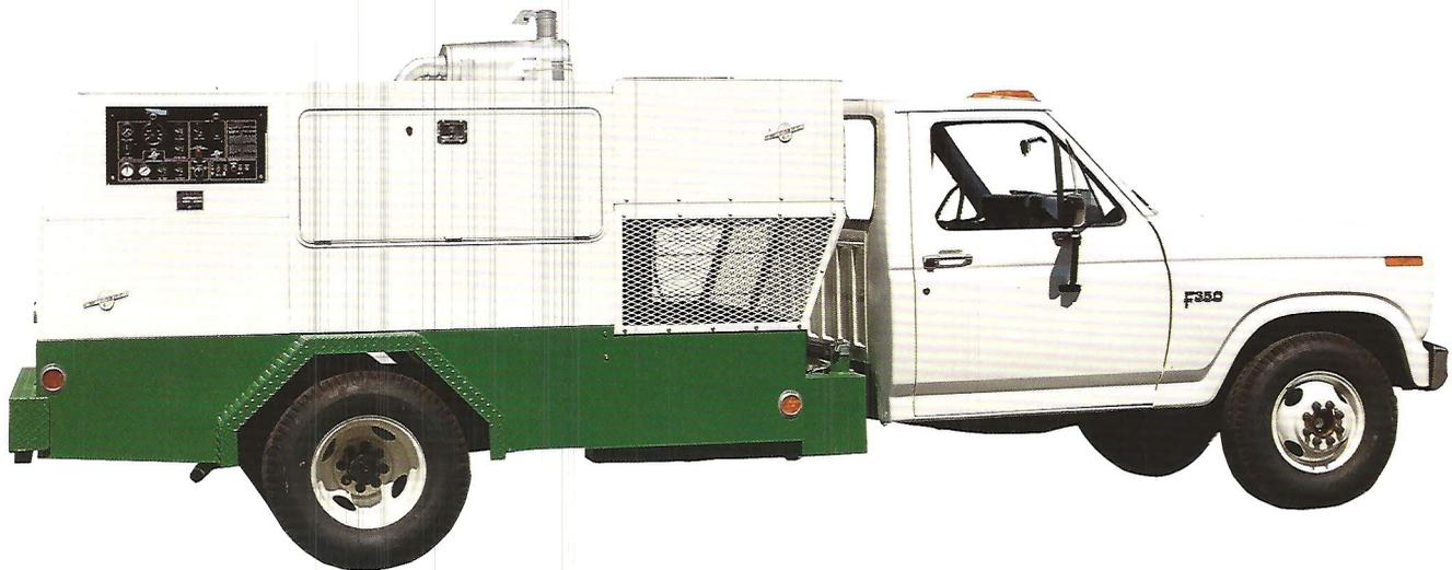
*Designed to start all standard body aircraft (except the B-757 and re-engined DC-8), this 120 PPM machine is compact, dependable and competitively priced.*
